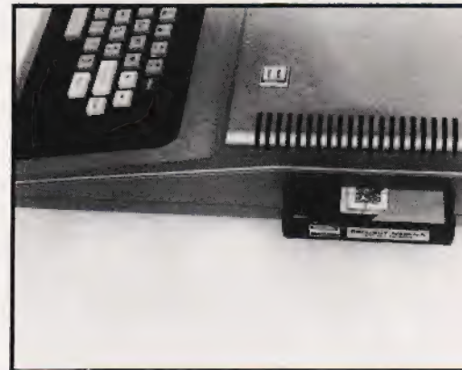
Above: Plugging in the Program Paks requires care — they can sometimes jam.
